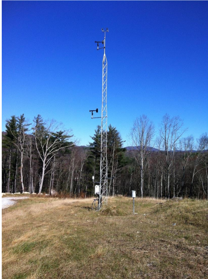
Figure 7. A mesonet station in North Carolina with nearby obstructions (trees).
