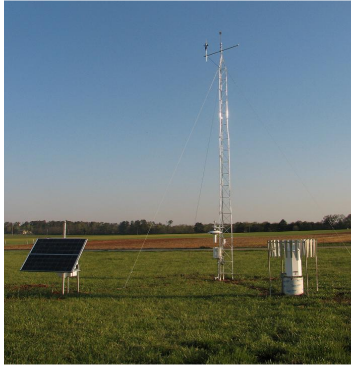
Figure 3. A mesonet station in Kentucky with good exposure.
