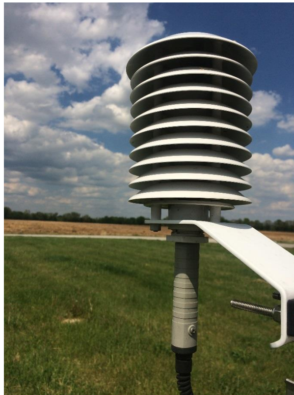
Figure 4a-b. a) Aspirated radiation shield, and b) Gill radiation shield (naturally ventilated).
